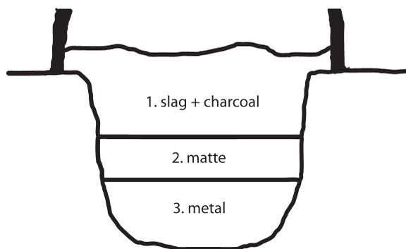
Fig. 2. A simplified diagram, showing the three resulting phases of an ideal copper-sulfide smelt: 1, silicate slag; 2, copper-rich matte (molten copper sulphide); 3, copper metal (adapted from Thornton et al. 2009, fig. 1).
