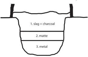
Fig. 2. A simplified diagram, showing the three resulting phases of an ideal copper-sulfide smelt: *1*, silicate slag; *2*, copper-rich matte (molten copper sulphide); *3*, copper metal (adapted from Thornton et al. 2009, fig. 1).
